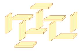
When electrolyte or polar solvent is added to the dispersion, the double layers are compressed. This allows the platelet edges and faces to more closely approach, resulting in a more rigid structure and consequently higher viscosity and yield value.
