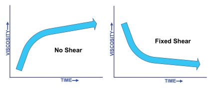
Smectite dispersions are also pseudoplastic, because increasing the rate of applied shear (thereby increasing structure breakdown) results in decreasing viscosities.
