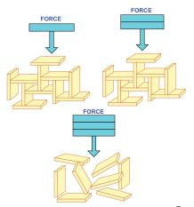
A unique and valuable feature of **VAN GEL®** Magnesium Aluminum Silicate and **VEEGUM®** Magnesium Aluminum Silicate clays is their ability to impart yield value at low viscosity. Stabilization of the dispersed phase is possible even in thin, fluid systems where flowability is important. Most common organic thickeners possess little or no yield value and can only stabilize suspensions, emulsions or foams at high viscosity.
