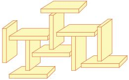
If the double layers become sufficiently compressed, face-face van der Waals attraction will predominate and the house of cards colloidal structure will be lost, as will thickening and suspending efficiency.
